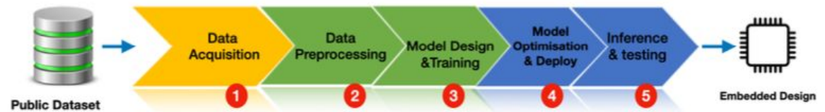
Figure 1: Workflow diagram of a TinyML project, including the deployment to an embedded device
