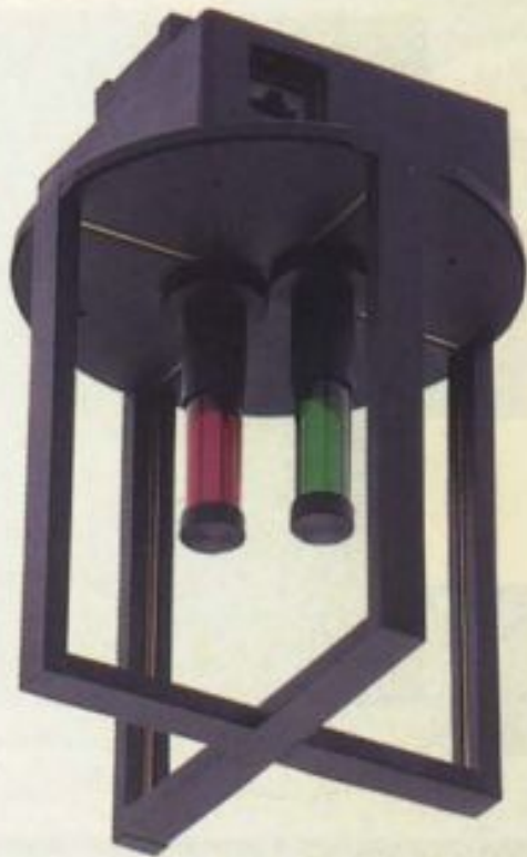
RADIO TRANSCIVER links pads and other movable computer devices to the wired network. This unit, intended to be mounted on the ceiling, contains antennas in its crossed arms and two light-emitting diodes to signal its status.
